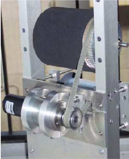
Detail of climber DC drive and mounted traction wheel
