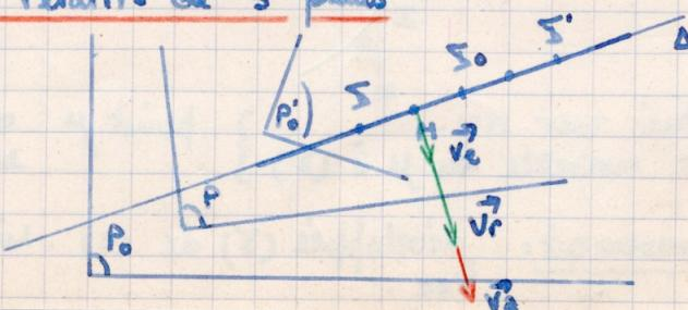
$$\left\{ \begin{array}{l} P/P_0 \rightarrow \Sigma' \\ P'/P \rightarrow \Sigma_0 \\ P'/P_0 \rightarrow \Sigma. \end{array} \right.$$
