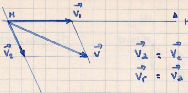
$$\begin{aligned} \vec{v}_2 &= \vec{v}_e + \vec{v}_r \\ \vec{v}_r &= \vec{v}_a - \vec{v}_e \end{aligned}$$
