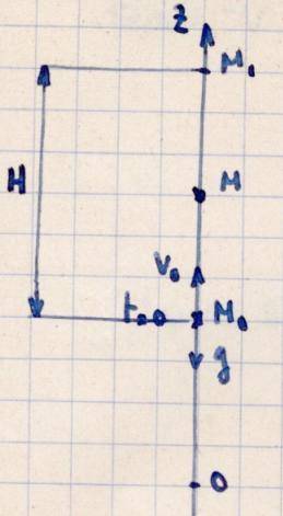
$$\left\{ \begin{array}{l} x = -gt \\ v = -gt + v_0 \\ h = -\frac{1}{2}gt^2 + v_0t + h_0 \end{array} \right.$$
