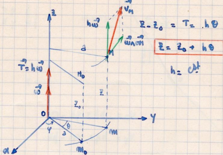
$$M \left\{ \begin{array}{l} x = a \cos(\theta + \varphi) \\ y = a \sin(\theta + \varphi) \\ z = z_0 + h \theta \end{array} \right. \quad \left\{ \begin{array}{l} \varphi = 0 \\ z_0 = 0 \\ z = h \theta \end{array} \right. \quad \left\{ \begin{array}{l} x = a \cos \theta \\ y = a \sin \theta \\ z = h \theta \end{array} \right.$$
