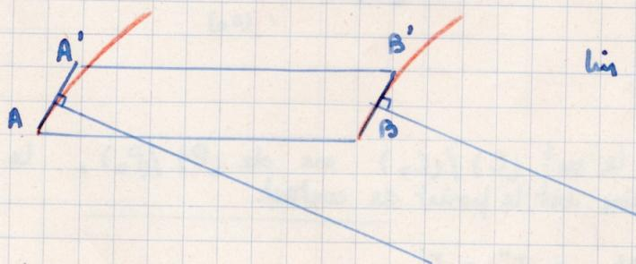
$$\lim_{\Delta t \rightarrow 0} \frac{\vec{AA'}}{\Delta t} = \lim_{\Delta t \rightarrow 0} \frac{\vec{BB'}}{\Delta t} = \vec{J} = \text{trav. instantanée.}$$
