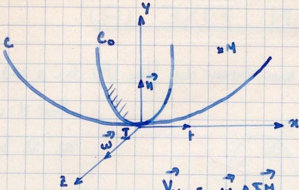
$$|\vec{v}_S| = \omega k \rightarrow \left( \frac{1}{k} = \frac{1}{R_0} - \frac{1}{R} \right).$$
