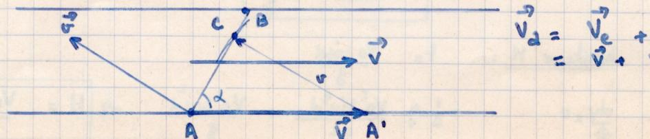
$$\begin{aligned} \vec{v}_d &= \vec{v}_e + \vec{v}_r \\ &= \vec{v} + \vec{v}_r \end{aligned}$$
